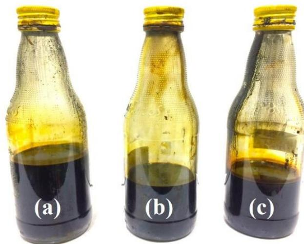
**Fig. 7** Fuel from plastic waste (a) PE (b) PP (c) HDPE.
