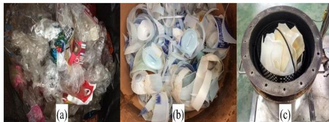
Fig. 1 Plastic waste samples (a) PE, (b) PP and (c) HDPE.
