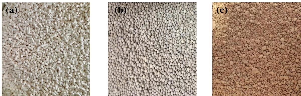
Fig. 2 The catalyst, (a) ZSM-5, (b) dolomite, and (c) kaolin.
